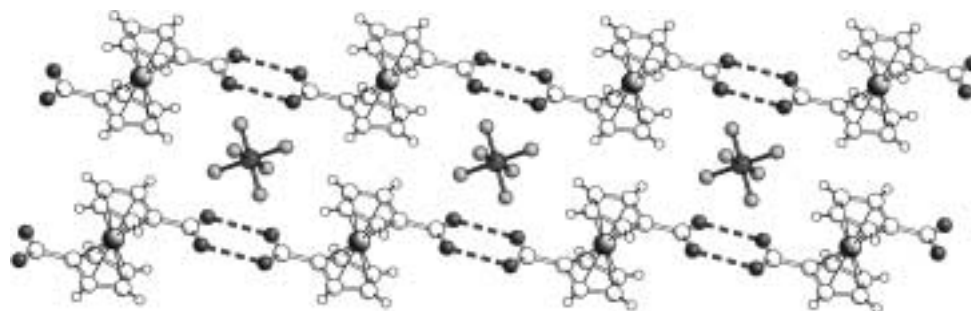
Figure 1. Parallel cationic \{[(\eta^5\text{-C}_5\text{H}_4\text{COOH})_2\text{Co}^{\text{III}}]^+\}_n chains form a step-ladder two-dimensional superstructure with the [\text{PF}_6]^- anions accommodated in between the steps and interacting with the cyclopentadienyl ligands through charge-assisted \text{C-H}^{\delta+} \cdots \text{F}^{\delta-} interactions.
